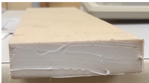
Fig. 3. Drying sample with silicone layer
