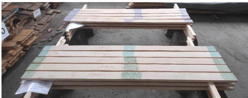
Figure 5. Two drying cages (green with no spiral grain), (blue with spiral grain)
