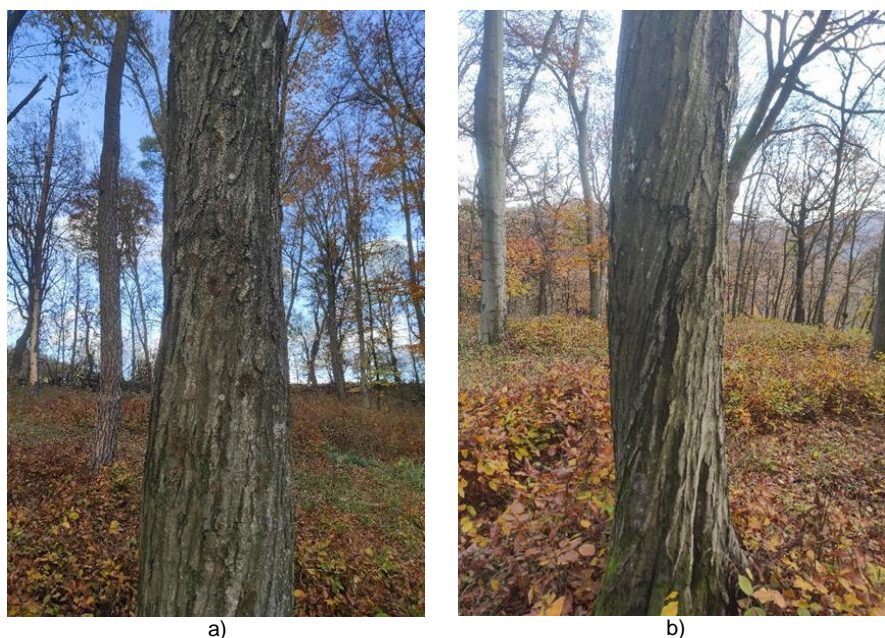
Fig 1. Selected samples in the forest a) with no spiral grain, b) with spiral grain
